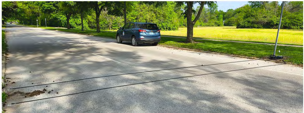
Figure 1 Traffic Counter Installation
